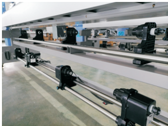
It can print whole roll with 3.2m width material, especially suitable for the production of high-precision inkjet cloth. Two rolls 1.27m width material can be printed at the same time (air-expansion shaft feeding & collecting system can be choose for the special textile material)
